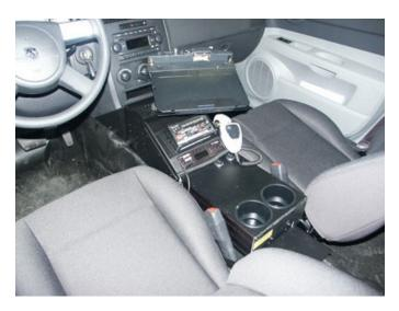
Route wiring and install emergency controls and accessories
